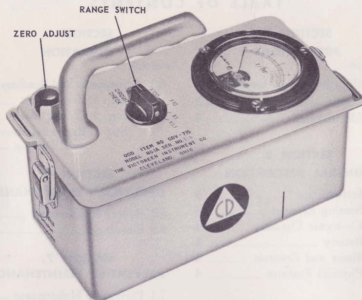
Figure 1. View of CD V-715, Showing Operating Controls
